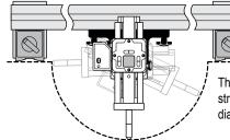
The measuring principle is the same for both long and short stroke bracket. The probe rod is very easily adapted to each diameter with extensions of different length.
