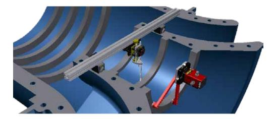
Before measuring, please check that you have mounted the bracket and probe correctly. If the bracket has been mounted skewed, the values will be incorrect. Image below show a linebore measurement, but the same principle apply to turbines.
